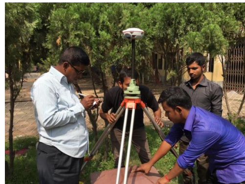
Figure-4: Total Station Survey using RTK-GPS Technique
