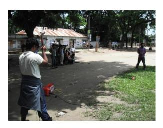
Figure 2.18 MASW Field Data Acquisition
