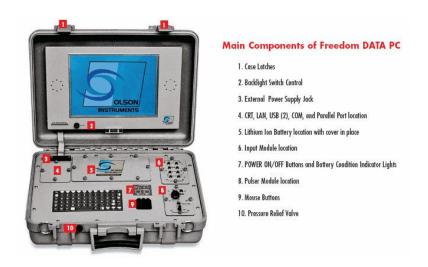
Figure 2.2 Main Component of the Freedom Data PC
