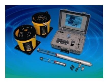
Figure 2.14 Freedom Data PC with P-SV Downhole Source and 1 Tri-axial Geophone Receiver used in Crosshole Seismic Investigations
