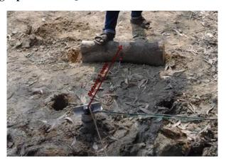
Figure 2.5 To set the wooden plank 1.0 meters from a borehole
