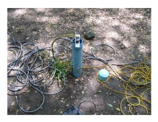
Figure 2.9 Make sure that the air bag at the geophone works. Then, put the geophone into the borehole and fix the safety rope with the holder
