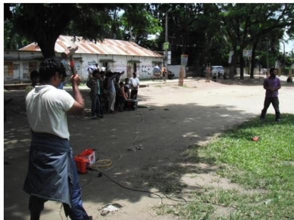
**Figure 2.18 MASW Field Data Acquisition**
