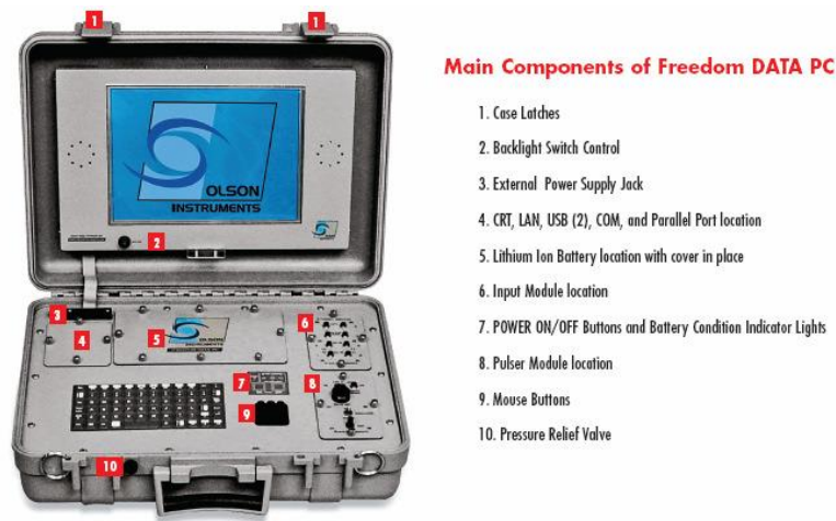
Figure 2.2 Main Component of the Freedom Data PC
