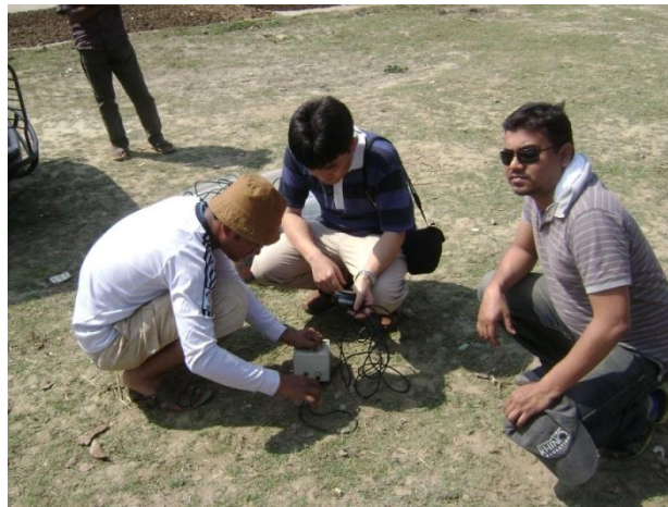
Figure 2.24 Field data acquisition of Single microtremor
