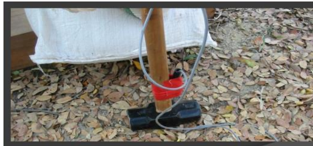
Figure 2.6 To attach the trigger to a hammer.
